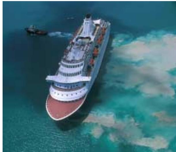
This cruise ship photographed from the air shows the huge plumes of silt stirred up as it is taken away from the dock. Ship traffic in Bermuda's harbours cause regular impacts through re-suspension of bottom sediments. The industrialisation of Bermuda's harbours has caused significant declines
